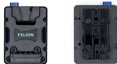
NANOLNP-C Dimension: 88.5(L)mm*62(W)mm*46(H)mm Weight: 141g Features: Suitable for 7.4V DC Output on NP-F Plate, D-Tap Output: 10-16.8V
