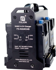
FX-NANO4S - NANO 4-Channel Charger Output: 16.8V / 2.0A (CH 1+2 / CH 2+4) Power Draw: 80W Dimension: 160(L)mm*93(W)mm*124(H)mm Features: charges NANO batteries Weight: 743g
