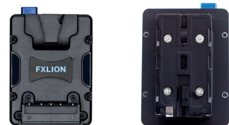
NANOLNP Dimension: 88.5(L)mm*62(W)mm*46(H)mm Weight: 123g Features: for using Nano V-Mounts with Sony NP-F Battery plates, D-Tap Output
